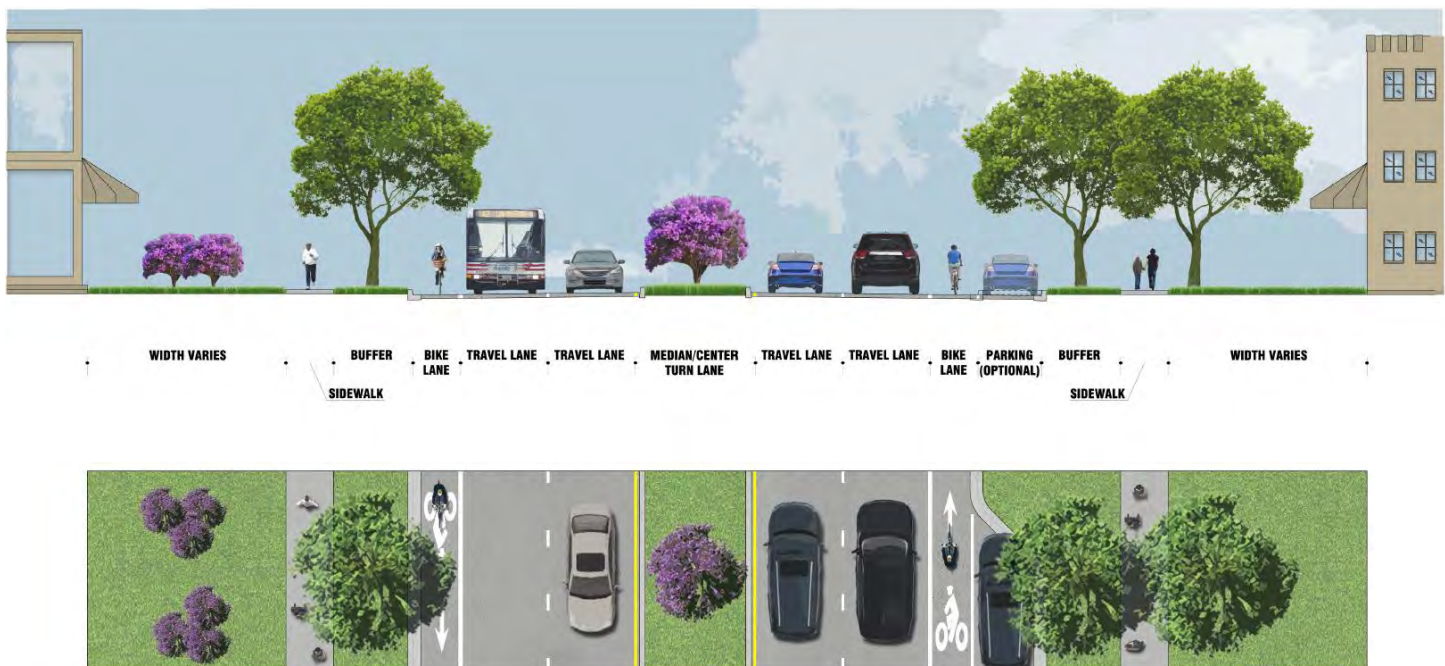
FIGURE 27. TYPICAL REGIONAL BOULEVARD CROSS SECTION
